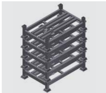
These dismantlable pallets are endowed with a removable storage frame.
